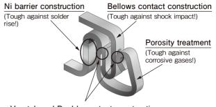
V notch and Double contact constructions
